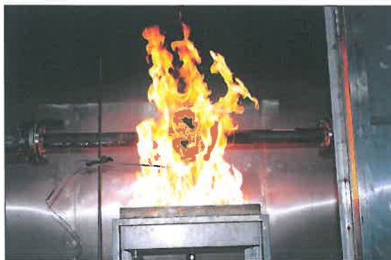
[Photo 3] Fire endurance test
