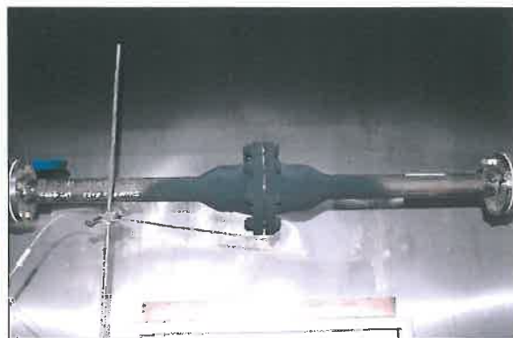
[Photo 4] Hydrostatic tightness test
